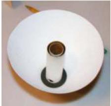
(*Optional*) **Strengthen the Booster Joint:** Using CA glue, soak the outside of the Booster Coupler. Once thoroughly dry, it will need to be sanded to fit into the Sustainer. That can be done at the end of construction.
