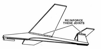
**26** Apply glue reinforcements to the wing, stabilizer and hook joints. Reinforce by applying a thin line of glue to the joint, then smoothing it out with your finger tip.
