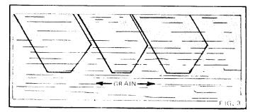
Cut out the fins with a sharp modeling knife or single edge razor blade. Sand the sides of the fins until smooth. Sand until smooth and round all edges except the root edge (the edge which will be attached to the body). Sand the root edge of each fin so it is square and flat.
