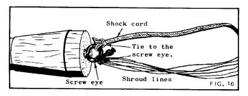
☐ 16. Install the nose cone on the front of the payload section. Connect the shock cord, parachute and screw eye as shown in fig. 16. Push the parachute into the body tube, packing the shroud lines and shock cord in over it. Push the base of the adapter into the forward end of the body tube.
