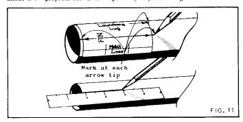
☐ 11. Cut out the fin spacing guide from the pattern sheet. Wrap it around the upper stage body at the end with the engine mount unit as shown. The alignment marks on the pattern should match perfectly. Mark the body at each of the arrow points, remove the guide and draw a straight line connecting the corresponding pairs of marks. Mark the booster body tube in the same way.
