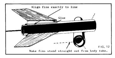
☐ 12. Apply glue to the root edge of one of the upper stage fins. Attach the fin to the upper stage body tube with the edge of the fin exactly on one of the lines made in step 11. Align the fin so it projects straight away from the body tube. Following the same procedure, attach the other two upper stage fins and the booster fins. Do not set either stage on its fins while the glue is wet.
