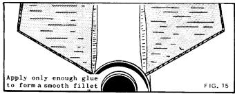
□ 15. When the first glue on the fins has dried, apply a fillet of glue to each of the fin-body joints and to the launch lug support as shown. The fillets should be smooth and free of bubbles. Support the rocket horizontally while the glue dries.
