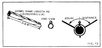
□ 13. Cut the launch lug stand-off dowel to the same length as the launch lug. Apply a line of glue to one side of the lug and press the stand-off into place on the glue. Make sure the two pieces are perfectly parallel. After the glue has set a few minutes, apply glue to the other side of the stand-off and attach the unit to the upper stage mid-way between two fins so the rear of the lug is 1-1/4" ahead of the front of the fins. Be sure the unit runs parallel to the body tube.
