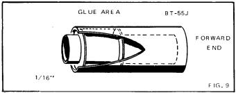
9. Smear glue around the inside of the BT-55J booster body tube to cover an area 1" deep at one end. Insert the engine mount unit, with the end that projects farthest first, into the booster body tube until the rear ring is 1/16" inside the tube as shown. Be especially careful to make this assembly exactly as the illustration shows. The rocket will not operate properly if any error is made in positioning.
