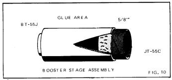
10. Apply glue to the inside of the forward end of the booster body tube to a depth of 5/8". Slide the remaining stage coupler into the end of the tube so that 5/8" of the coupler is inside the body and about 5/8" projects forward. Wipe away any excess glue.
